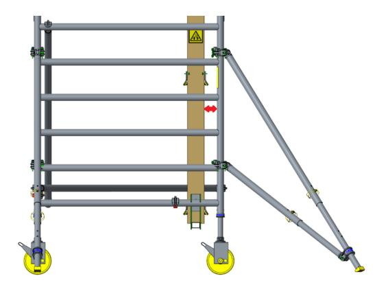
4. Connect the guide rail to the rung. Make sure there is 11cm of space between the upright of the scaffold and the tube of the coupling (see red arrow in the image above). Also make sure that the rail is neatly vertical, use a spirit level if necessary. Note: If you are only going to place 1 platform on the upper level and plan to lift the panel over the handrail, keep 40cm for this distance.
