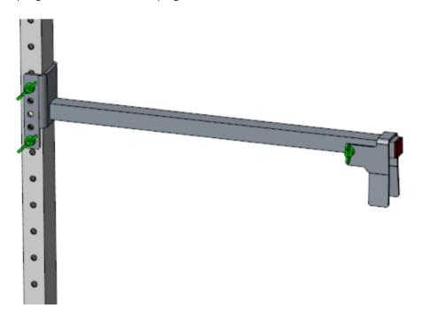
2. Check the position of the top beam in relation to the top of the panel. If necessary, adjust this position by means of the adjustment holes so that the beam hangs just above the top of the panel.
