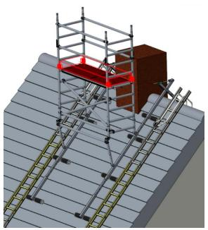
13. Place the toe board brackets and toe boards, creating a complete work platform.
