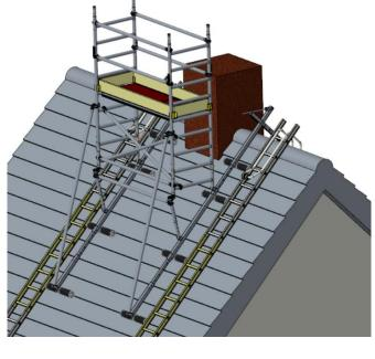
15. The chimney scaffold is ready for use. Access the platform by stepping under the platform on the chimney side and climbing up via the inside of the scaffolding. The platform can be entered through the hatch in the platform.
