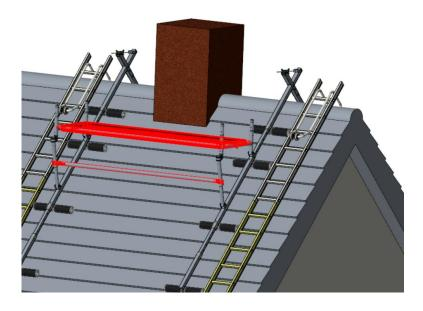
8. Place the platform without hatch onto the two horizontal rungs of the base frames. Slide the wind protection locking pins under the load-bearing rungs.
