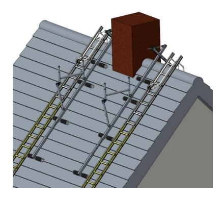
7. Place the extensions at the bottom of the base frames. Make sure that they are adjusted to the maximum length. Secure them at the correct position with a locking pin.
