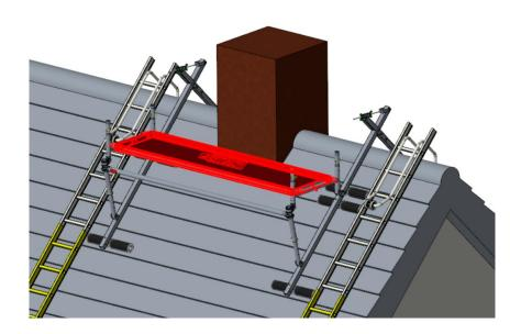
7. Place the platform on the two horizontal rungs of the two base frames. Slide the wind protection locking pins under the load-bearing rungs.
