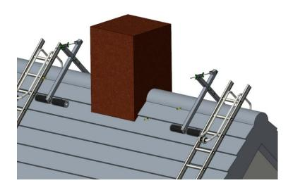
2. First, place the Chimney Access Ridge Stand (CARS Unit) on the ridge of the roof. Depending on the actual dimensions of the roof and the roof tiles used, it should be possible to support the support rollers on the second row of roof tiles. This is to avoid damage to the ridge tiles and the first row of roof tiles at all times. Adjust the Chimney Access Ridge Stand (CARS Unit) with the butterfly nut so that the Chimney Access Ridge Stand (CARS Unit) has the same angle as the roof.
