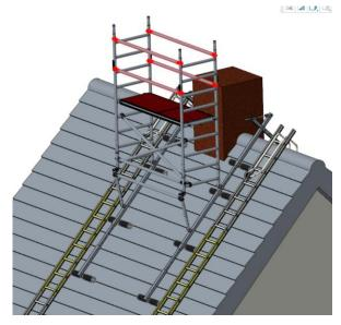
12. Place the other 4 horizontal ledgers on each side of the platform at knee and hip height. Make sure that the openings of the claws point outwards.
