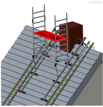
11. Place the platform on the 4th rung of the 8-stage frames. Slide the wind protection locking pins under the load-bearing rungs.
