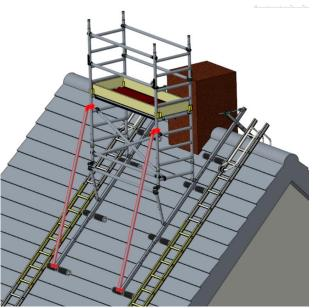
14. Finally, place the two girders between the lower eye of the two extensions and the two 8-stage frames. This provides additional stability while using the scaffolding. Should the coupling of the girder end up exactly at a rung, adjust the extension so that this problem no longer occurs.
