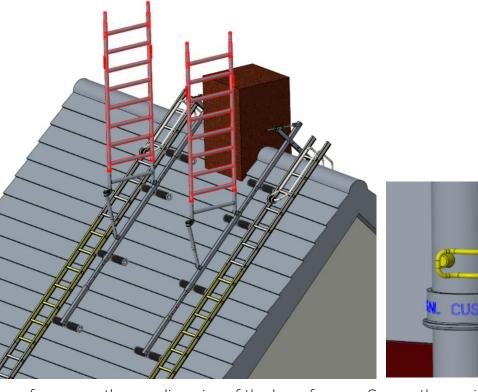
8. Place the 8-stage frames on the coupling pins of the base frames. Secure these with locking pins.
