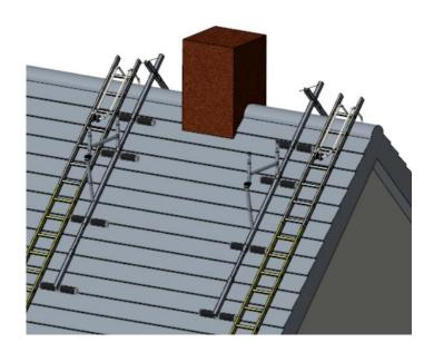
7. Place the extensions on the bottom of the base frames. Make sure that they are adjusted to the maximum length. Secure them at the correct position with a locking pin.
