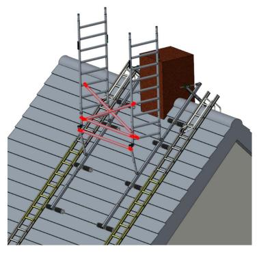
9. Place a horizontal just above the rung of the base frame. Make sure that the openings of the claws point outwards.
