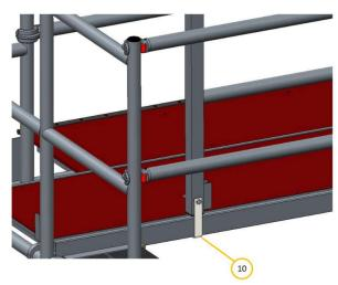
10. Put the connector around the platform profile and firmly fix the butterfly nut.
